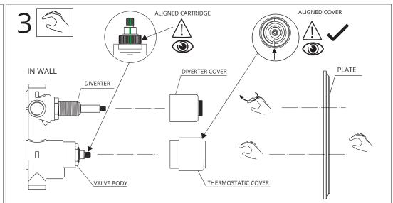
**NOTE**: Make sure that the green line on the cartridge is aligned. Put inside covers like image n.3 Put thermostatic knob with button facing upwards like image n.4 and screw it in.
